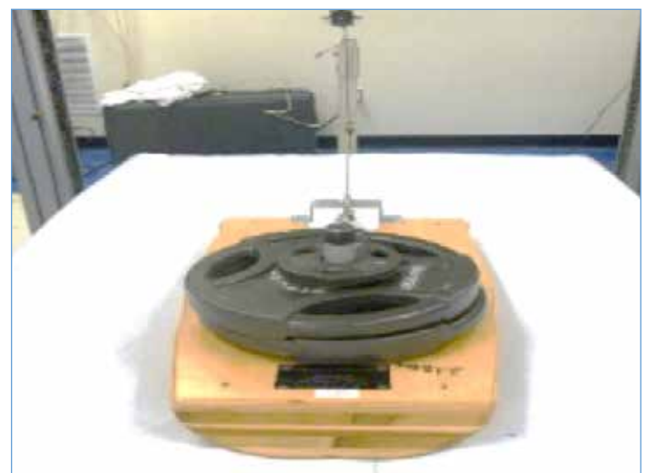
Figure 4: Horizontal Stiffness Test. A pelvic-shaped device is placed in the seat section and pulled 10 mm toward the foot of the bed. The resulting pushback force, a measure of shear, is recorded at 0, 1, 2, 3, 4, and 5 minutes after the motion.
